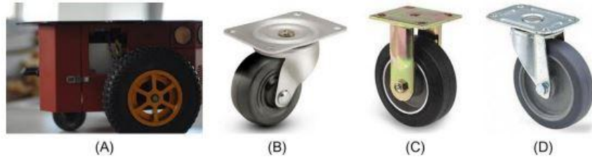
Figure 2.2. Conventional wheel types: (A) fixed wheel, (B) castor wheel, (C) powered steering wheel without offset, (D) powered steering wheel with longitudinal offset.
