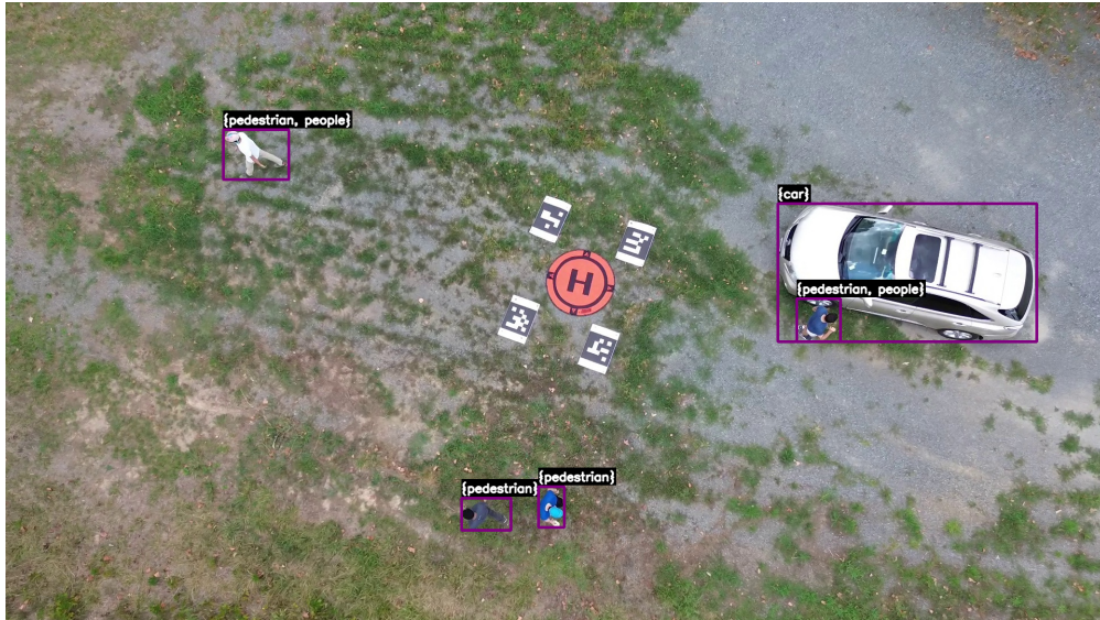
(b) Set predictions obtained from performing inference on a single frame from the UAS flight test data. Some of the objects have predictions that are the same as the point predictions of Figure 6a, while two of the detected objects are assigned classification sets from the CP.
