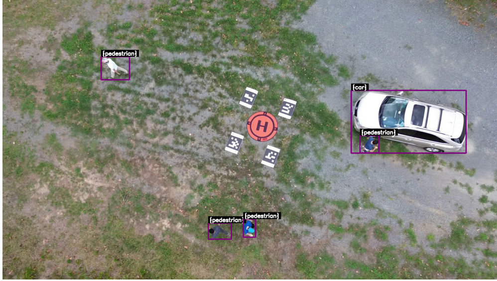
(a) Point predictions obtained from performing inference on a single frame from the UAS flight test data. All the objects were successfully detected with the correct classifications in the frame.
